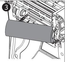
Insert the ink ribbon into the holder, right side first. Slot left hand side of the ribbon into the teeth on the left.
