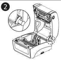
A lock located at the rear of the cover engages with the lower section, holding the cover open.
