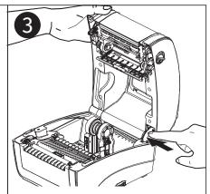
To close the cover, pull the upper cover slightly backwards and release the lock from the lower section. Gently close the cover.
