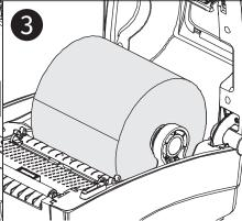
Position the roll between the mounts and ensure that the bearings engage with the roll core. Secure the roll by pressing down on the media holder lock.
