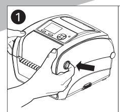
Open the upper printer cover by pulling the levers on each side forwards, then raise the cover as far as it will go.
