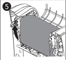
Rotate the winding gear until the plastic lead tape has been firmly wound and the black portion of the ribbon has reached the printer head. Close the ink ribbon cover and upper cover.
