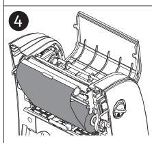
Use a piece of adhesive tape to attach the ribbon to the winding roller and insert the roller into the winding mount.
