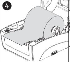
Take the paper, with the printable side facing up, and pull it up through the media sensor, then place the front edge onto the cylinder.
