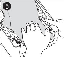
Adjust the media guide width by rotating the media guide adjustment knob.
